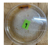
Water + Iron Day 19: The iron has rusted.
